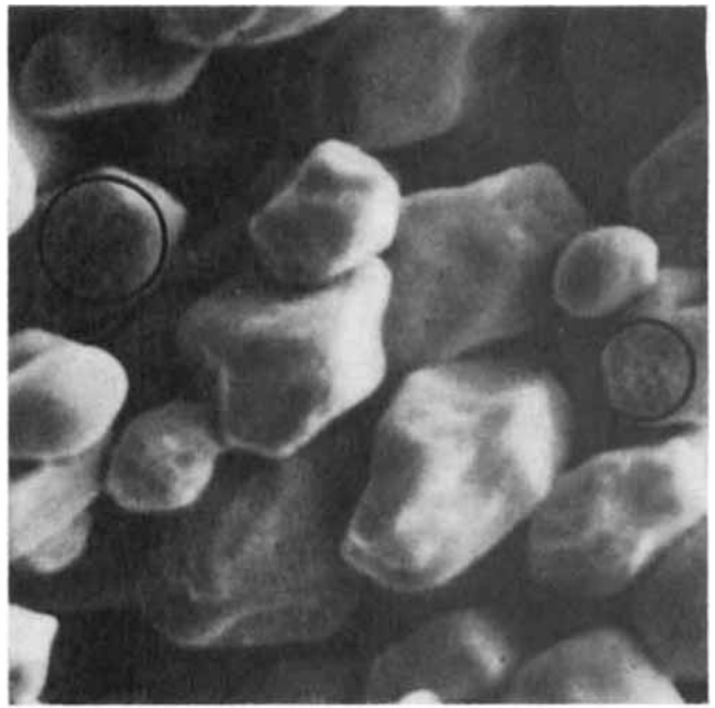
Figure 18 —Surface of cornstarch tablet compressed at 10,000 psig., photographed after addition of water (approximately 2300 \times ). Circled areas show "pitted" appearance of some grains.
